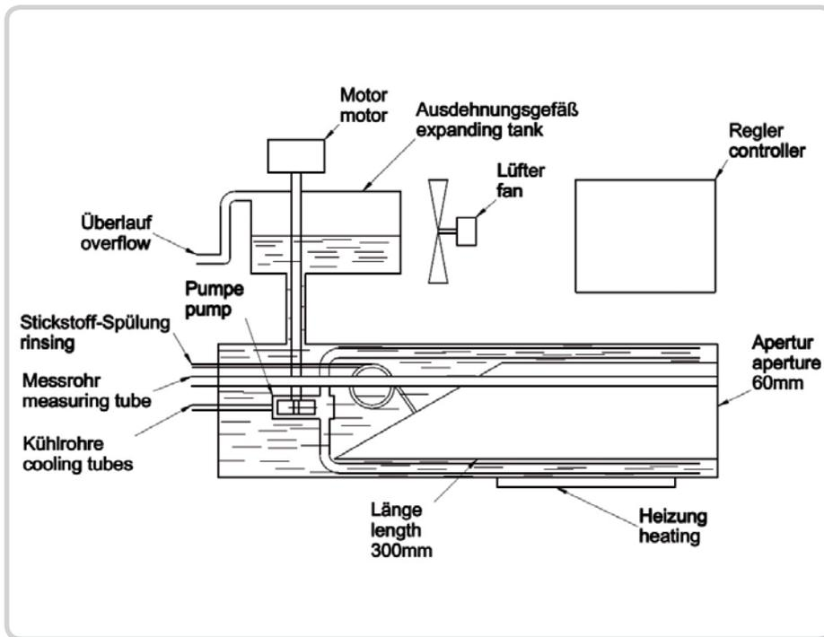
Figure 1: ME30 Blackbody Calibration Source (schematic presentation)
